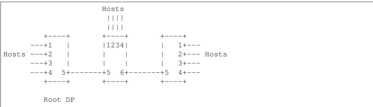
Non-root switches flood only to the root. The root switch reflects incoming floods back out. Non-root switches flood packets from the root locally and to switches further away from the root. Flooding is entirely implemented in the dataplane.
